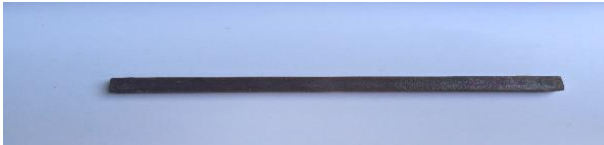
Fig 3: 15% Coconut shell powder and High-density polyethene (specimen for bending test)
