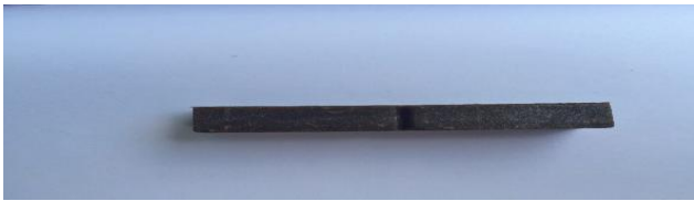
Fig 2: 10% Coconut shell powder and High-density polyethene (Specimen for impact test)
